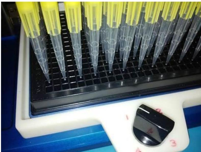
Now rotate the knob to **Position #2**, the microplate will then move to the adjacent empty well below the 96 channel tips to dispense into. Each position positively clicks in place without needing to align by hand.
