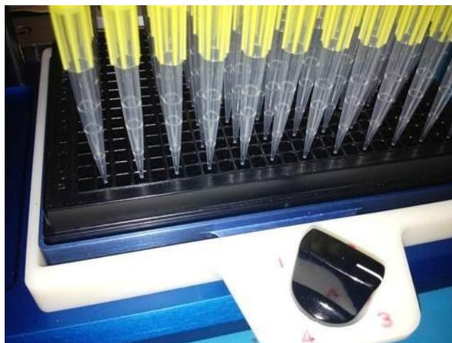
Finally rotate to **Position #4** to finish the 96 to 384 dispenses.
