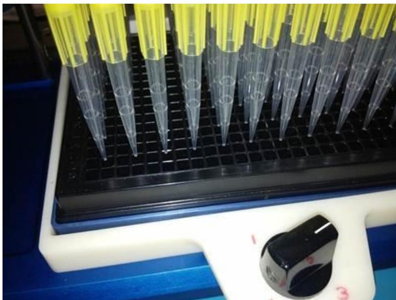
Again rotate the knob to **Position #3** and the plate is positioned in the well below. Each position positively clicks in place.
