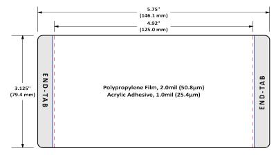
"For a more rigid easier-to-handle and apply film, check out SealPlate"
