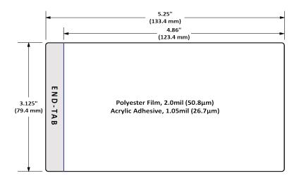
"For a dimensionally larger film with two end-tabs for ease of handling, check out SealPlate"
