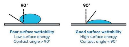
→ A smaller contact angle is better for the cell adhesion.
