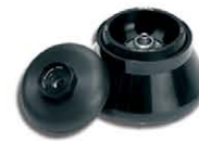
6 x 50ml rotor 21,000 rpm / 41,410 xg
